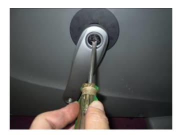
10. Use a slotted screwdriver to fix the cover (item #8 in the table) to the crank.
