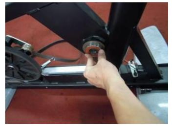
3. Slide the pedal axle set (item #1 in the table) into the frame from the right side.
