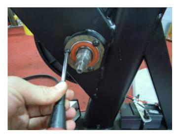
5. Install the 3 screws to secure the bearings on both sides.
