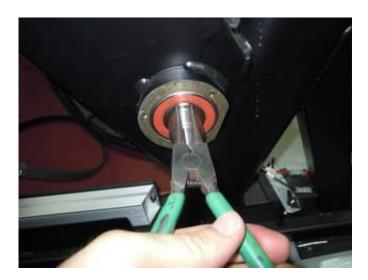
4. Install the snap ring (item #5 in the table) to secure the bearing on the left side of the frame.
